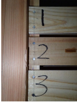
Figure 8. Details of the joint between wooden laths and supporting wood Figure 9. Compression test of plaster
