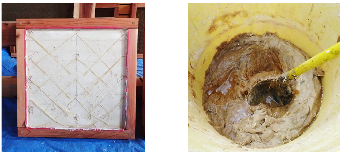
Figure 1. Construction of the specimen (left: after the 2nd layer coating, right: Plaster with hemp)
