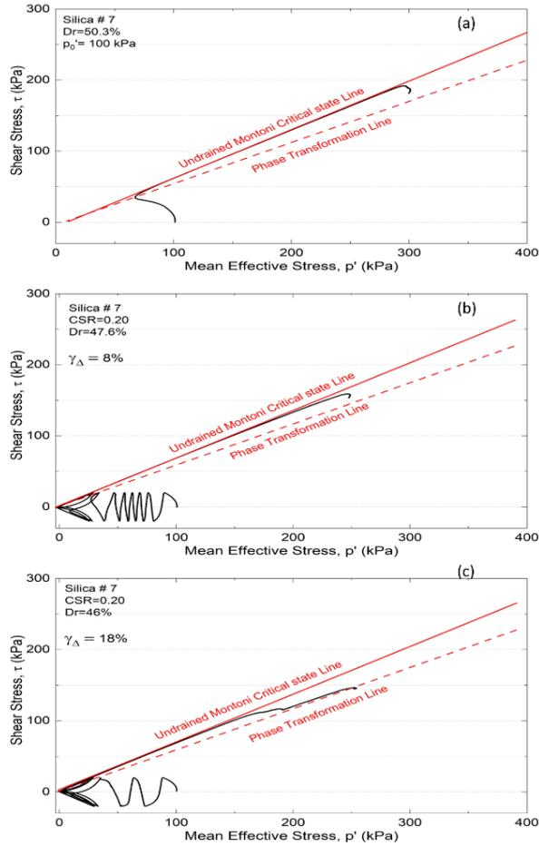
**Figure 10** Silica sand stress path showing the CSL at  $\gamma_{\Delta}=0,8$ , and 18%
