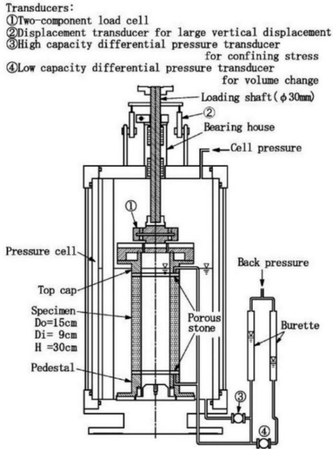
Figure 3. Torsional shear apparatus used in this study (Kiyota et al.<sup>10</sup>)
