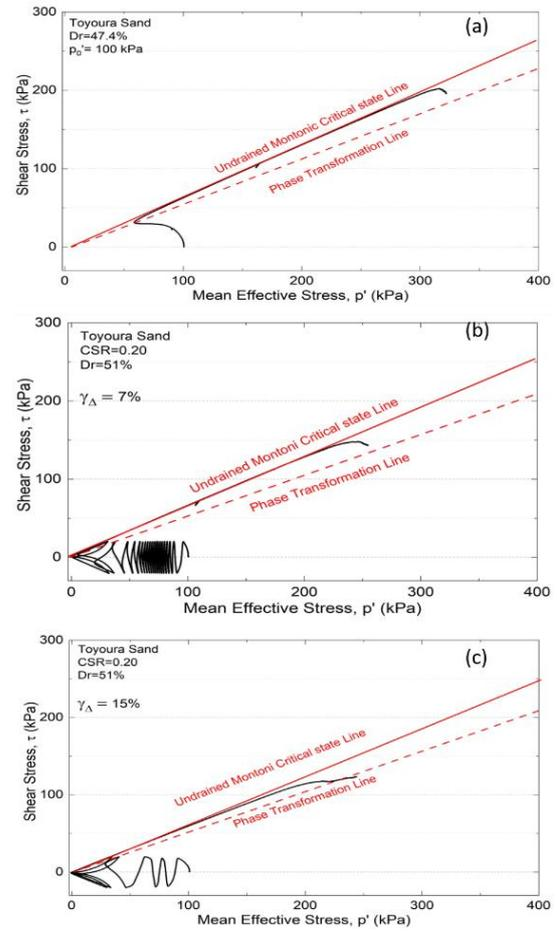
**Figure 11** Toyoura sand stress path showing the CSL at  $\gamma_{\Delta}=0,7$ , and 15%
