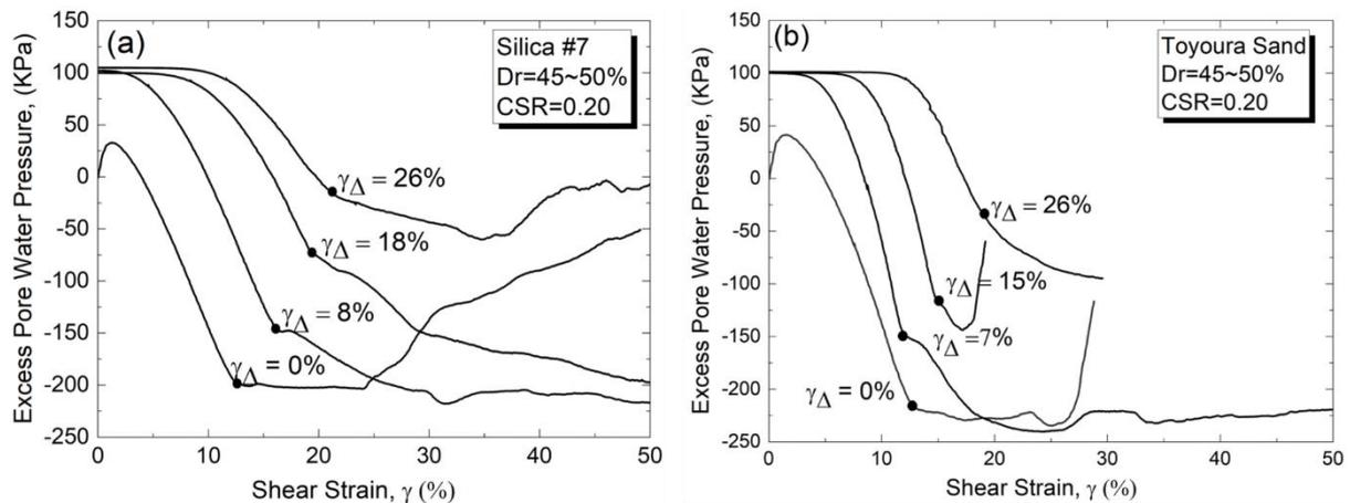
**Figure 7** Post-liquefaction EPWP response of sand in medium dense state ( $Dr=47\pm3$ ) for various shear strain level. (a) Silica #7 (b) Toyoura sand
