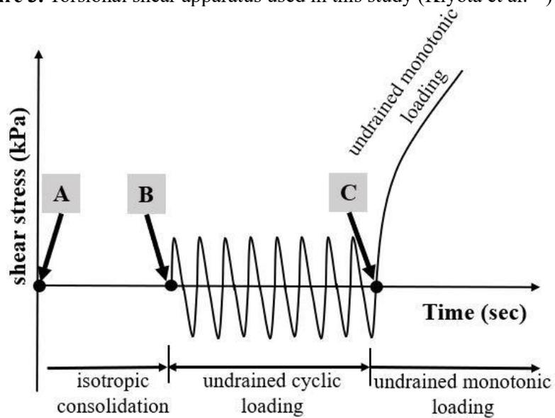
Figure 4. Test procedure to investigate post-liquefaction shear strength after Yasuda et al.<sup>14</sup>
