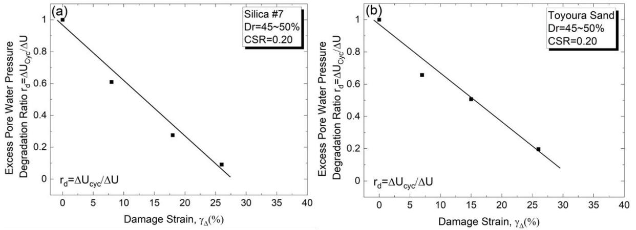
**Figure 13** Excess pore pressure degradation ratio versus damage strain (a) Silica #7 (b) Toyoura sand
