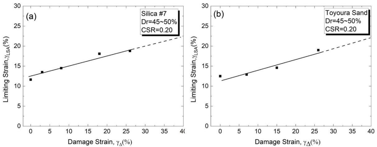
**Figure 9** Relationship between limiting strain and damage strain (a) Silica #7 (b) Toyoura sand
