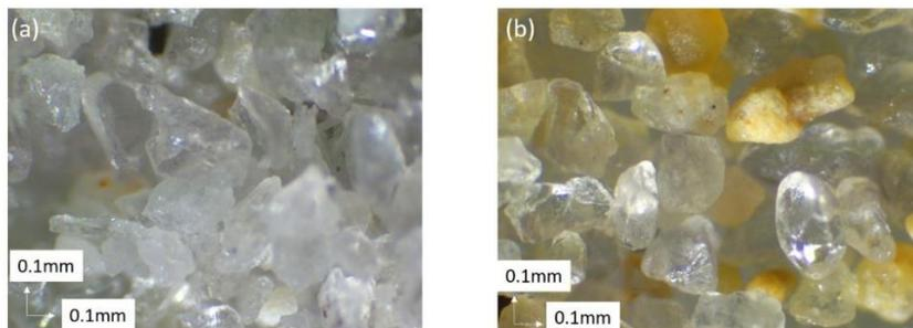
**Figure 1.** Microscopic picture with 4x optical zoom (a) Silica #7 (b) Toyoura sand
