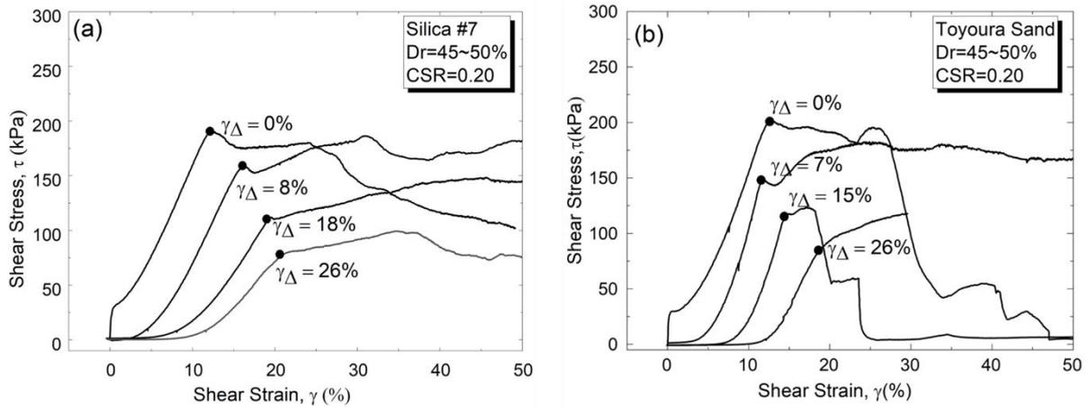
**Figure 6** Post-liquefaction stress-strain response of sand in medium dense state ( $Dr=47\pm3$ ) for various shear strain level. (a) Silica #7 (b) Toyoura sand
