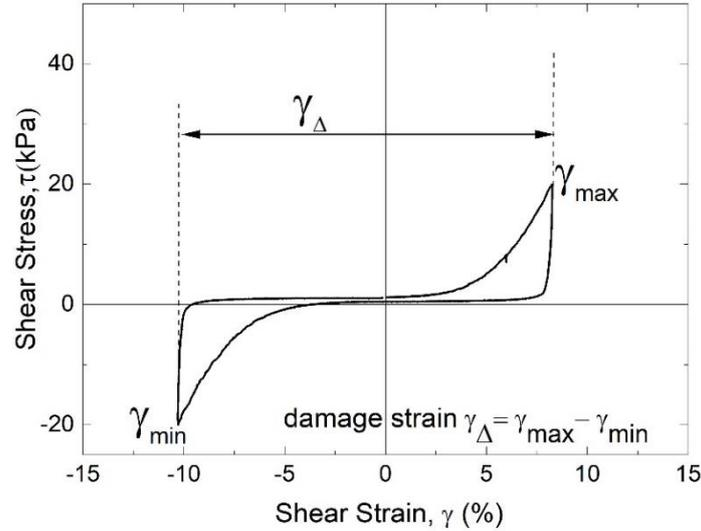
**Figure 5.** Schematic representation of damage strain
