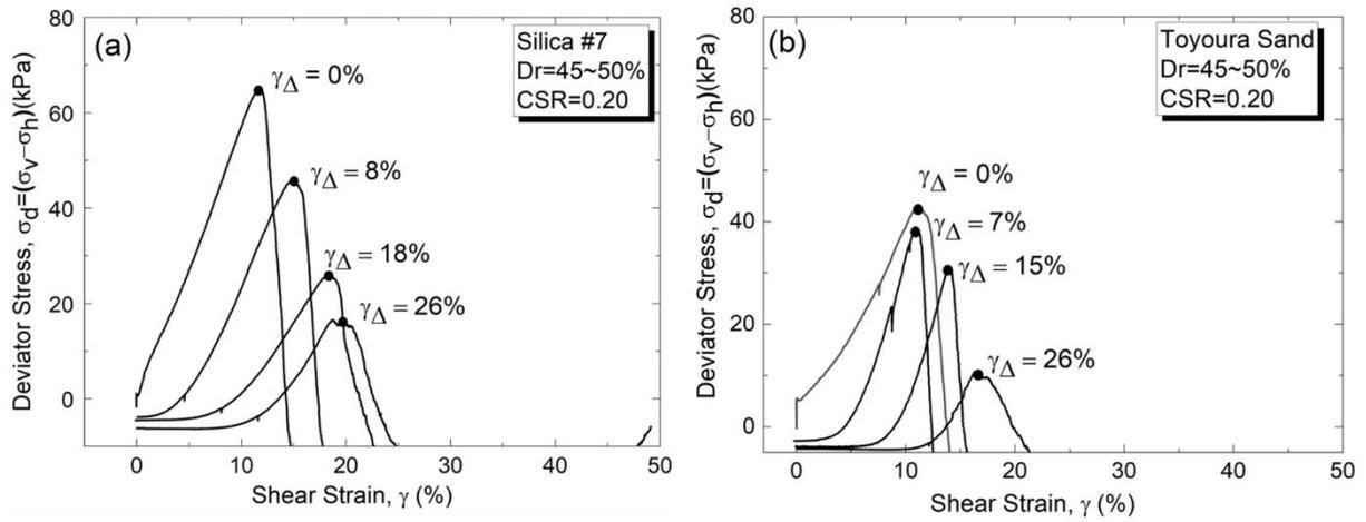
**Figure 8** Post-liquefaction Deviator stress -strain response of sand in medium dense state ( $Dr=47\pm 3$ ) for various shear strain level. (a) Silica #7 (b) Toyoura sand
