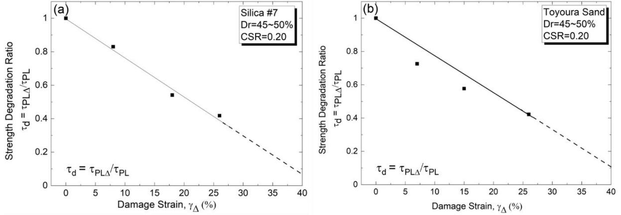
**Figure 12** Strength degradation ratio versus damage strain (a) Silica #7 (b) Toyoura sand
