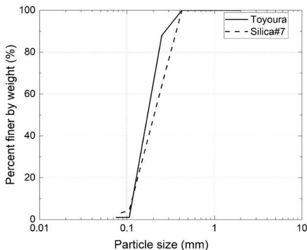
**Figure 2.** Particle size distribution of Silica sand No. 7 and Toyoura sand used in this study.
