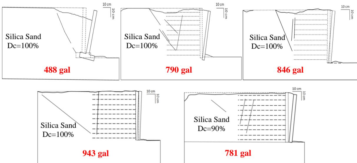
**Figure 4.** (a) T-shape RW, (b) Phosphor-bronze geogrid RS- RW, (c) TGS 700 geogrid RS-RW, (d) geocell RS-RW ( $D_c=100\%$ ), (e) geocell RS-RW ( $D_c=90\%$ )
