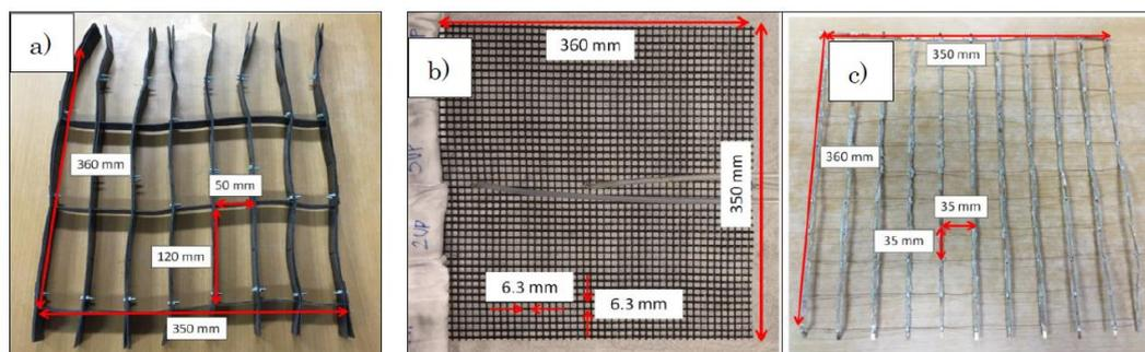
**Figure 3.** (a) Square-shaped geocell, (b) TSG 700 Geogrid, (c) Phosphor bronze geogrid
