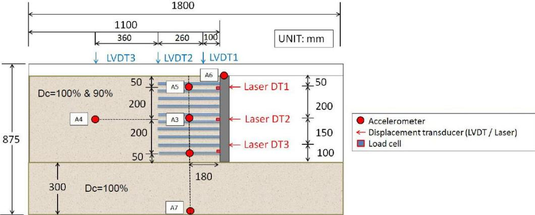
**Figure 1. Schematic diagram of GRS RW model**
