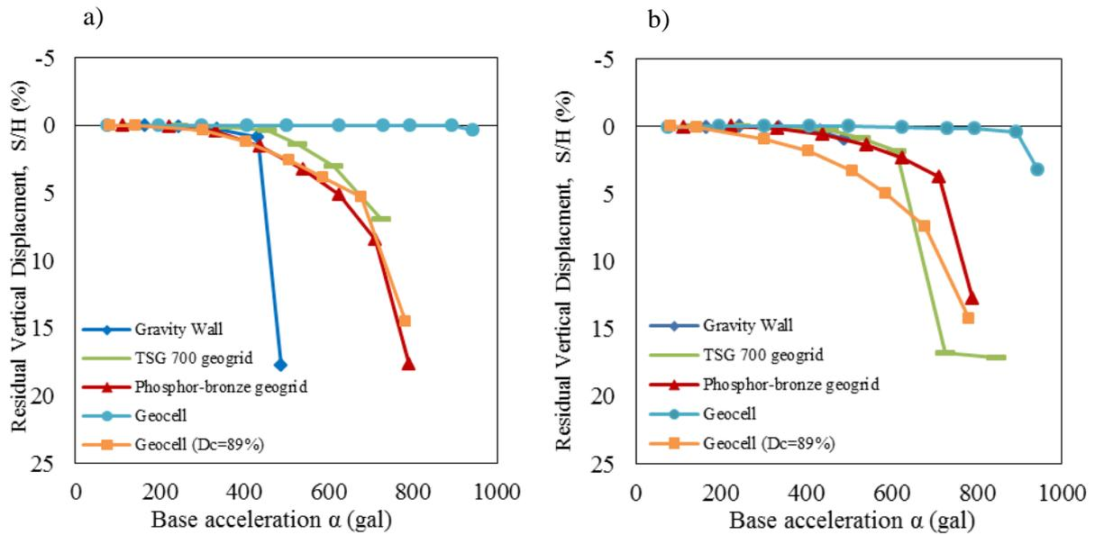
**Figure 6**, Backfill settlement at (a) 36 cm, (b) 72 cm
