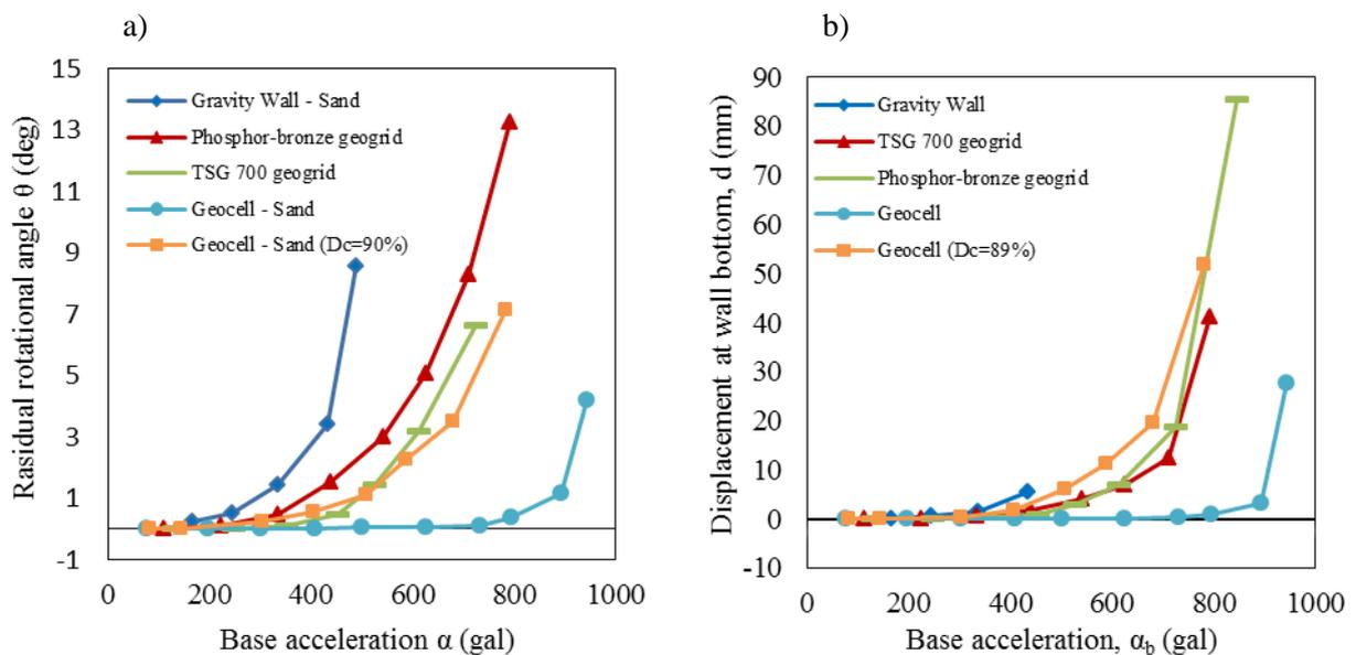
**Figure 5, (a) Residual rotational angle, (b) Wall bottom displacement**
