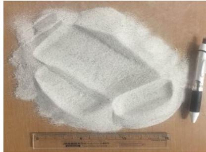
**Figure 2.** Silica Sand No.7 backfill material
