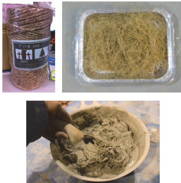
Figure 1. Abaca fiber before cut (left), after cut (middle), and mixed in mortar (right)
