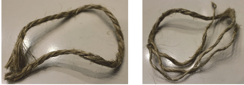
Figure 2. Abaca fiber in the form of Abaca rope before separation (left) and after separation (right)
