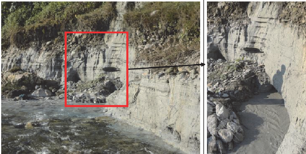
Figure 3 A muddy silty water outlet at bank of Kali River (Technical research report, 2014)
