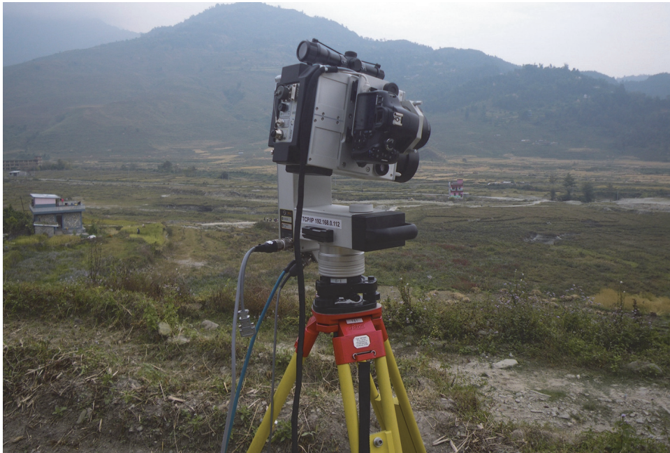
Figure 15 A LiDAR machine LPM-321, used for scanning survey area
