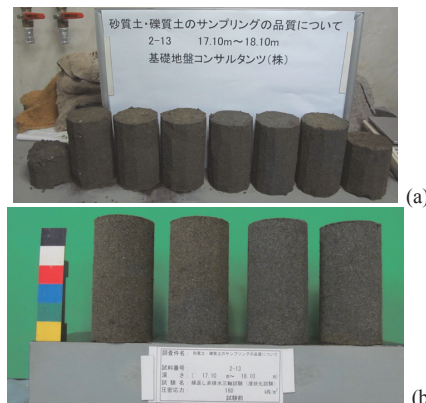
Figure 9 (a) Extruded samples of As2 sandy soil obtained by TS sampler; (b) samples after trimming
