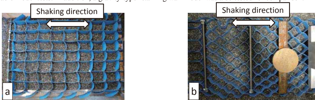
Figure 1. a) Square-shaped geocell model; b) Diamond-shaped geocell model
