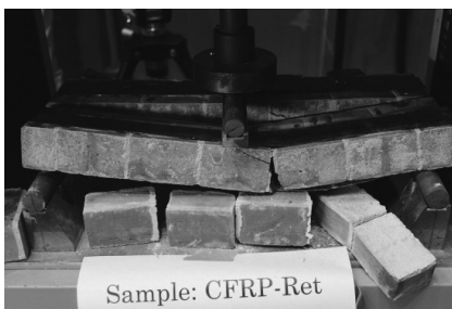
(c) Failure pattern of CFRP-retrofitted masonry wallet
