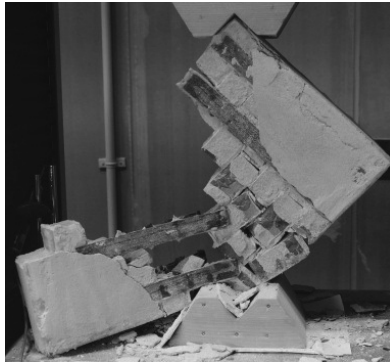
(c) Failure pattern of masonry wallet retrofitted with 0.0072 CFRP volumetric ratio with four strips on each face
