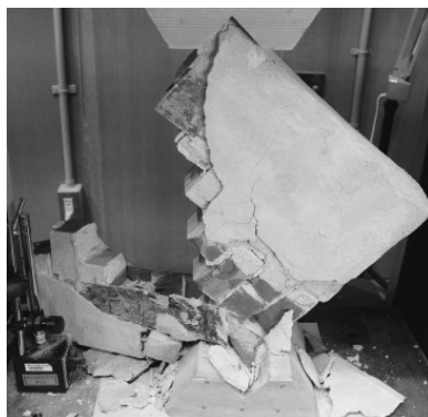
(a) Failure pattern of masonry wallet retrofitted with 0.0072 CFRP volumetric ratio with two strips on each face
