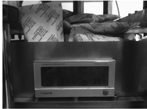
Fig. 6 Shear box covered by silica gel and temperature and humidity measurement
