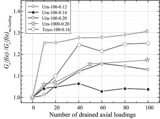
**Figure 8.** Relationship between  $G_s/f(e) / G_s/f(e)_{\text{no loading}}$  and number of drained vertical cyclic loading,  $N_c$
