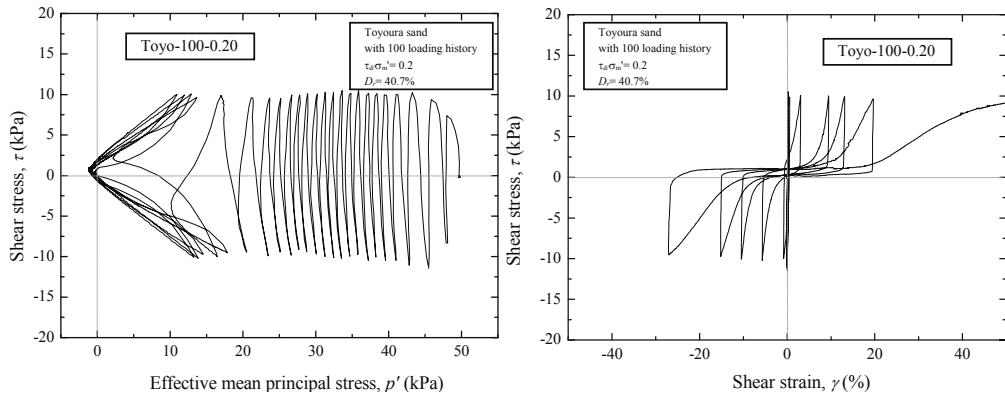
**Figure 13.** a) Effective stress path and b) stress-strain relation of Toyoura sand with 100 drained vertical cyclic loading history
