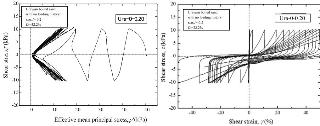
**Figure 9.** a) Effective stress path and b) stress-strain relation of Urayasu boiled sand without drained vertical cyclic loading history
