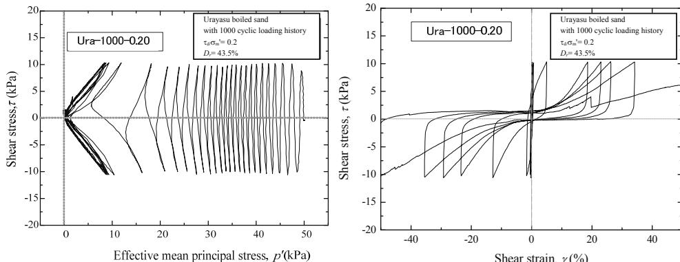
**Figure 11.** a) Effective stress path and b) stress-strain relation of Urayasu boiled sand with 1000 drained vertical cyclic loading history
