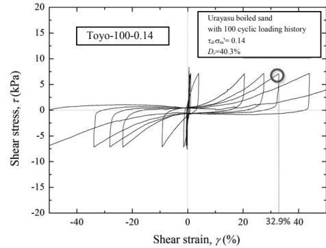
**Figure 16.** Stress-strain relation and limiting strain
