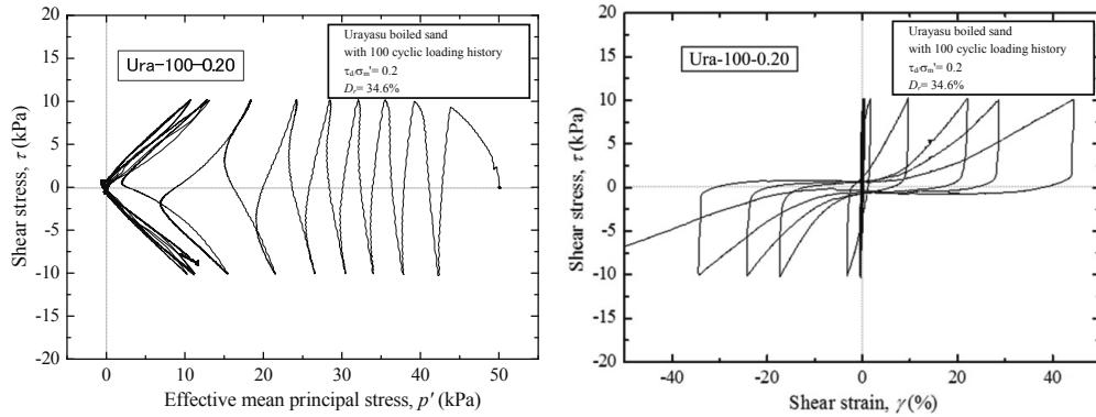
**Figure 10.** a) Effective stress path and b) stress-strain relation of Urayasu boiled sand with 100 drained vertical cyclic loading history
