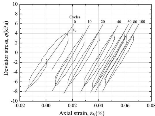
**Figure 4.** Relationship between deviator stress and axial strain during drained vertical cyclic loading before liquefaction test
