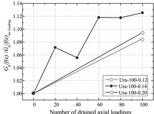
**Figure 6.** Relationship between  $G_d/f(e) / G_d/f(e)_{\text{no loading}}$  and number of drained vertical cyclic loading,  $N_c$
