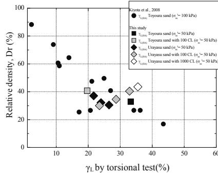
**Figure 17.** Relationship between limiting shear strain and relative density
