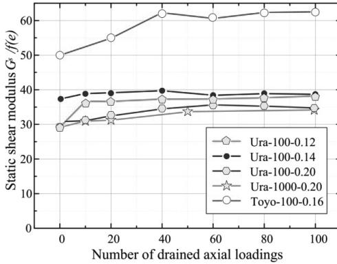
**Figure 7.** Relationship between  $G_s/f(e)$  and number of drained vertical cyclic loading,  $N_c$
