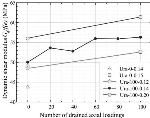
**Figure 5.** Relationship between  $G_d/f(e)$  and number of drained vertical cyclic loading,  $N_c$
