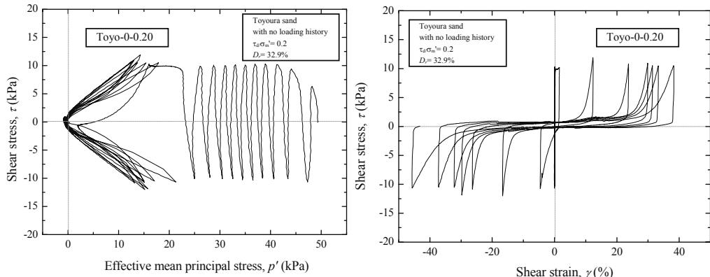
**Figure 12.** a) Effective stress path and b) stress-strain relation of Toyoura sand without drained vertical cyclic loading history
