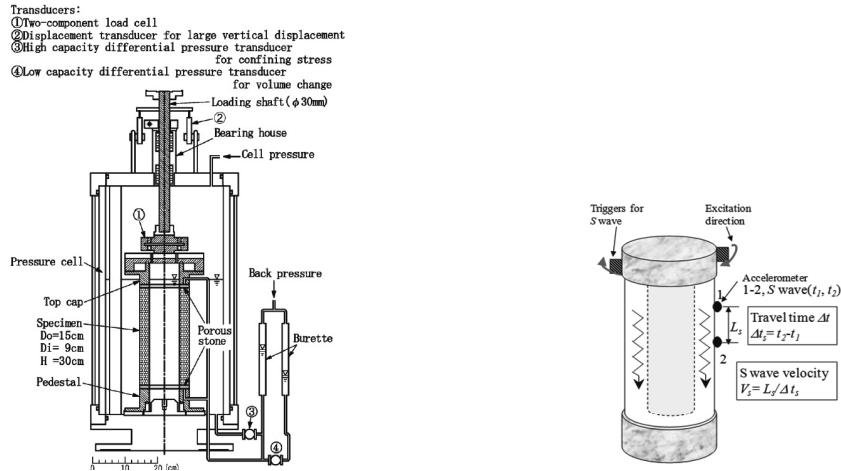
**Figure 2.** Torsional shear test apparatus
