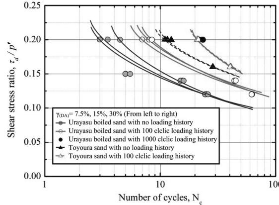
**Figure 14.** Shear stress ratios required to cause double amplitude shear strain of 7.5%, 15% and 30%
