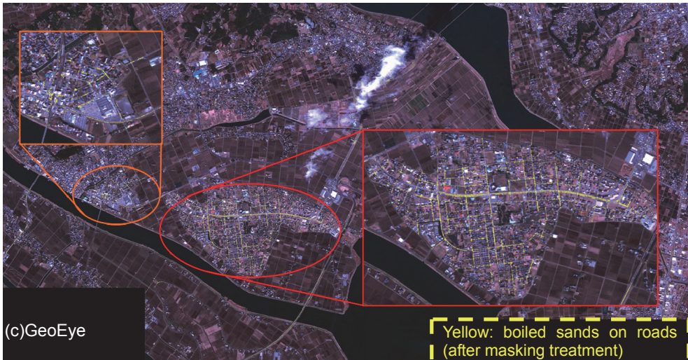
Figure 4 Result from analysis using training data of typical sand boiling for classification
