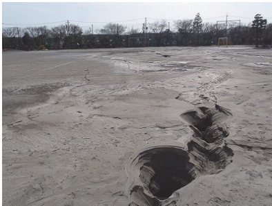
(a) Sand blows lined up in school ground Photo by Konagai K., on March 19 th at 35.638933, 139.895619
