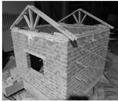
2. Securing holes using the straw during model construction
