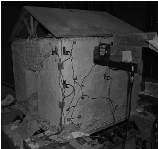
Figure 14. Retrofitted model after Run 48
