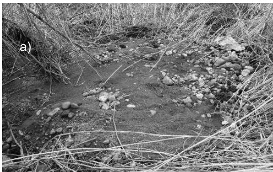
Photo 3. Boiling of gravelly soil at toes of Kokai river dike in Chikusei city, Ibaraki Prefecture (site Z)
