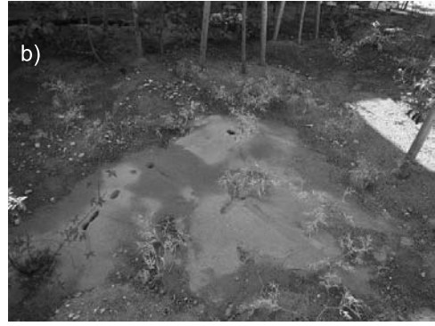
Photo 1. Extensive sand boiling a) at rice paddy in Toride city, Ibaraki prefecture (site C) and b) at back yard of supermarket in Urayasu city, Chiba prefecture (site R)
