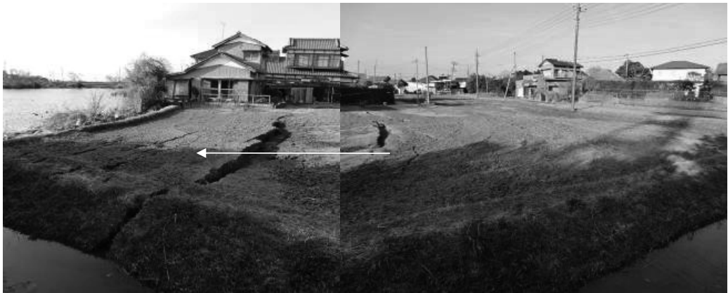
Photo 9. Lateral flow of level ground facing a pond in Katori city, Chiba prefecture (site L2)
