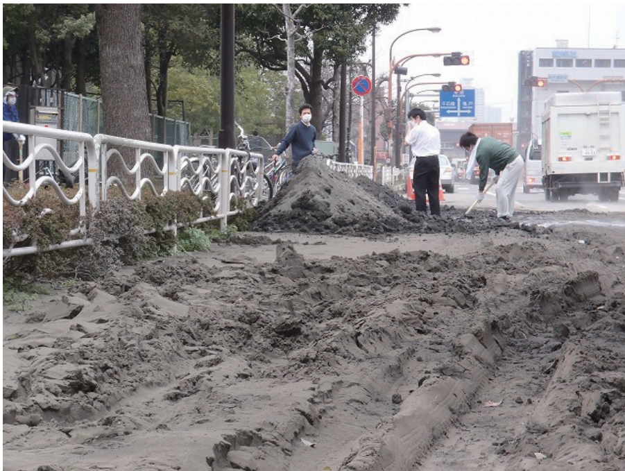
Figure 10 Liquefied sand near Shinkiba subway station (photo on 2011/03/15 by T. Kiyota. Location: 35.644812,139.828148)
