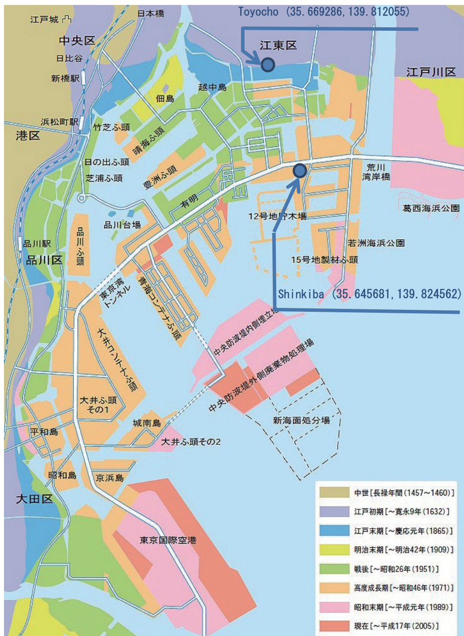
Figure 1 Locations of seismometers and times of landfilling (after “the history of Tokyo Port, MLIT”)
