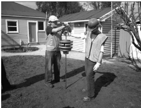
Photo 8 SWS test (Site 7 in Fig. 5). Behind of experimenters, there is house suffered from cracking.
