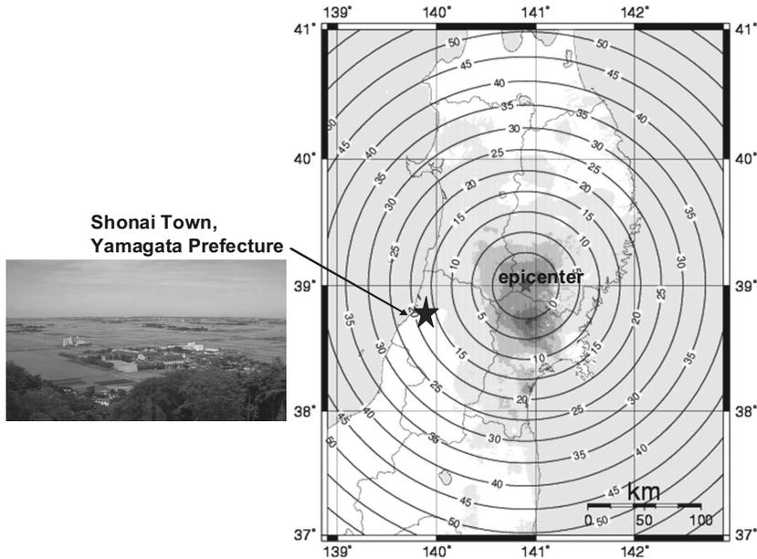
**Figure 2.** Epicenter and lead time between EEW and the arrival of strong tremors during the Iwate-Miyagi Inland Earthquake
