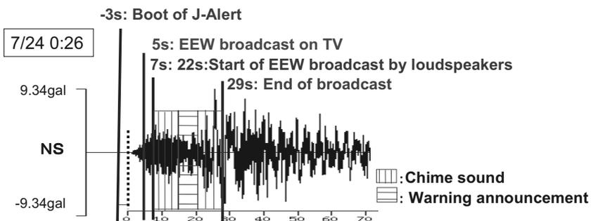
**Figure 4.** Timing of EEW broadcasting during earthquake on July 24
