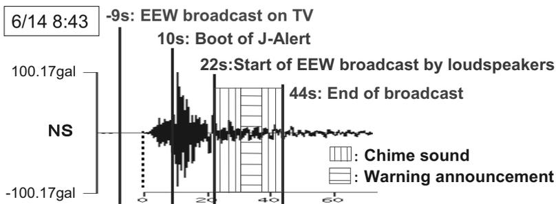
**Figure 3.** Timing of EEW broadcasting during earthquake on June 14
