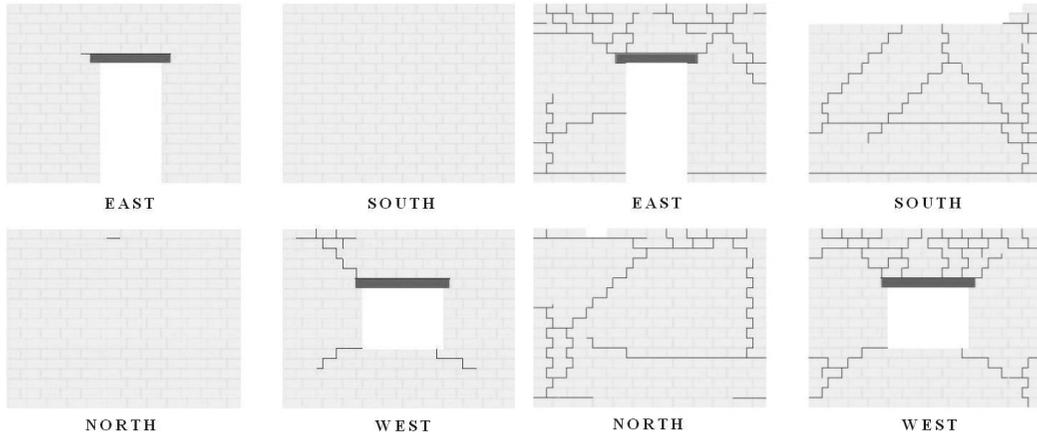
**Figure 5.** Crack patterns observed on non-retrofitted model after Run 22
