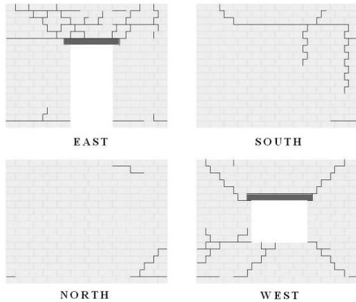
**Figure 9.** Crack patterns observed on for retrofitted model after Run 40
