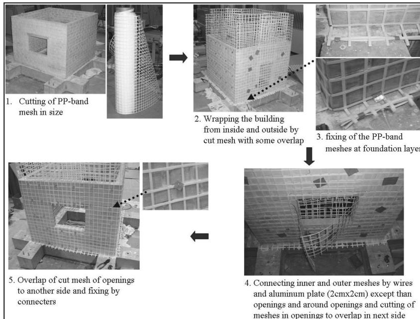
**Figure 2.** Retrofitting procedure
