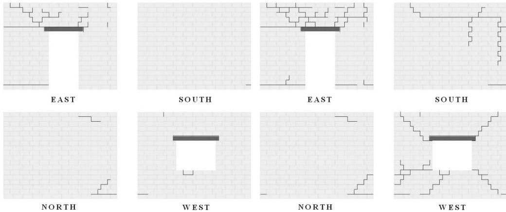
**Figure 8.** Crack patterns observed on retrofitted model after Run 22
