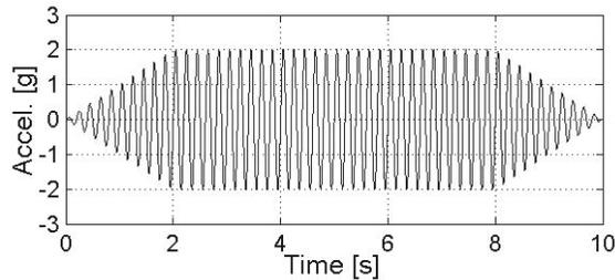
**Figure 3.** Typical Shape of Input Sinusoidal Motion
