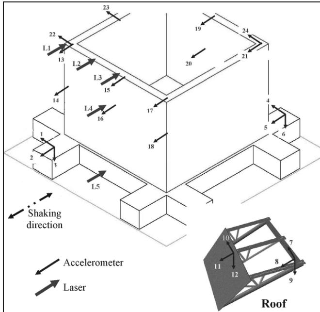
**Figure 4.** Location of accelerometers and lasers
