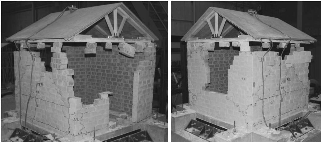
**Figure 7.** Non-retrofitted model after Run 45
