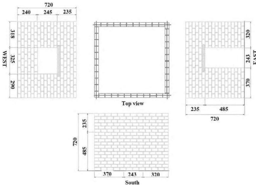
**Figure 1.** Model dimension (in mm)
