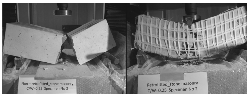
Figure 10. Failure pattern of stone masonry wallette (left: without retrofitting, right: with retrofitting)
