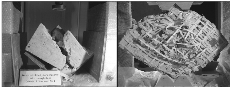
Figure 6. Failure pattern of stone masonry wallette (left: without retrofitting, right: with retrofitting)
