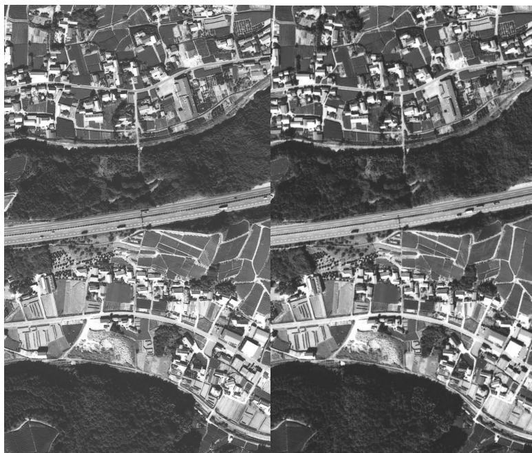
Fig. 5. Stereogram of the fill-section of the Tomei Express way in 1988 before the 2009 earthquake (Photos from Geographical Survey Institute of Japan). Latitude and longitude for the center of each photo: N34.75577°, E138.191614°, Width of each photo = 710m.
