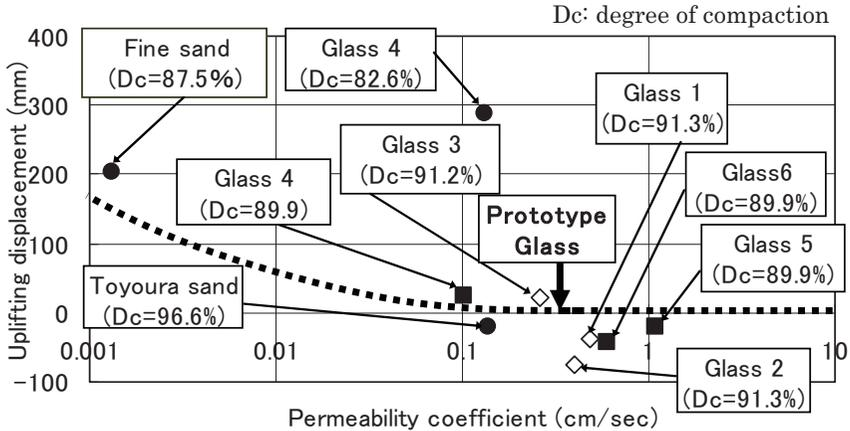
**Figure 5.** Relationship between uplifting displacement and permeability coefficient
