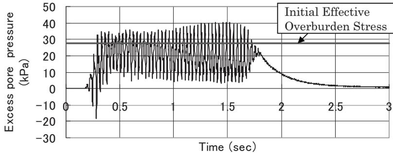
Figure 7. Time history of excess pore pressure (PP1, Glass 4, case 08-00)
