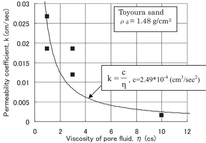
**Figure 3.** Relationship between permeability coefficient and viscosity of pore fluid
