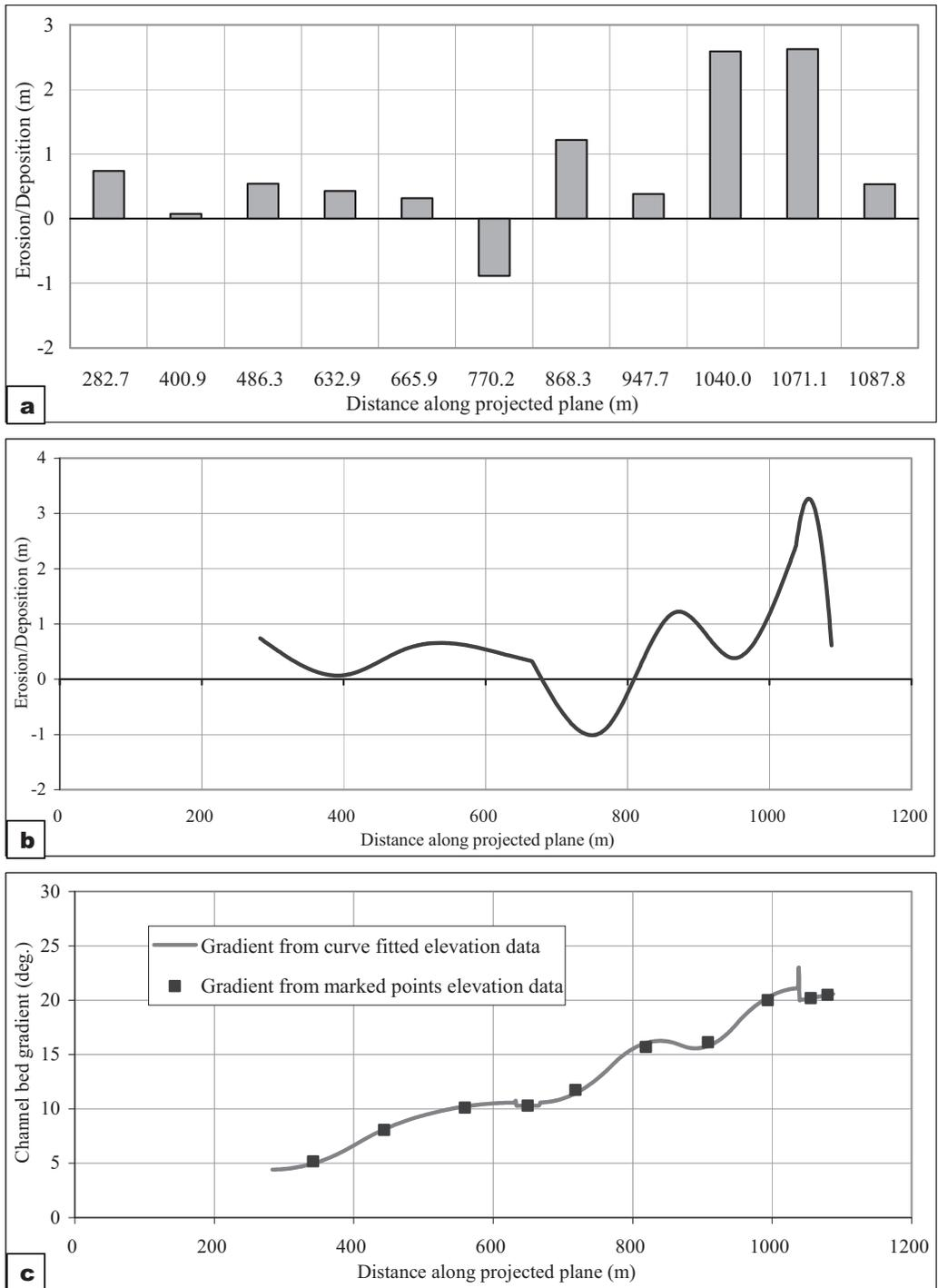
**Fig. 7: a)** Elevation changes of November measured points with reference to curve fitted to June measurement **b)** elevation changes along total length of nallah from curve fitted data **c)** nallah bed gradient
