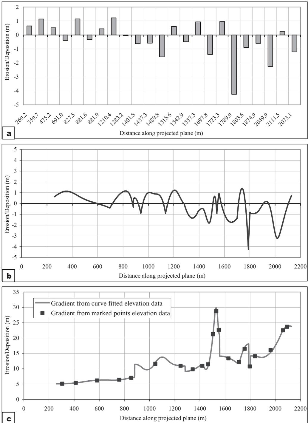
**Fig. 9: a)** Elevation changes of November measured points with reference to curve fitted to June measurement **b)** elevation changes along total length of nallah from curve fitted data **c)** nallah bed gradient
