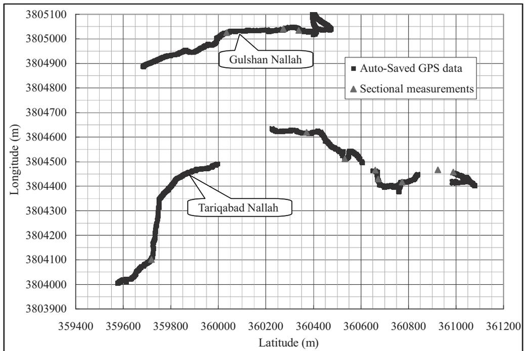
**Fig.11** Auto marked GPS data showing profiles of nallahs along with sections of velocity and discharge measurement
