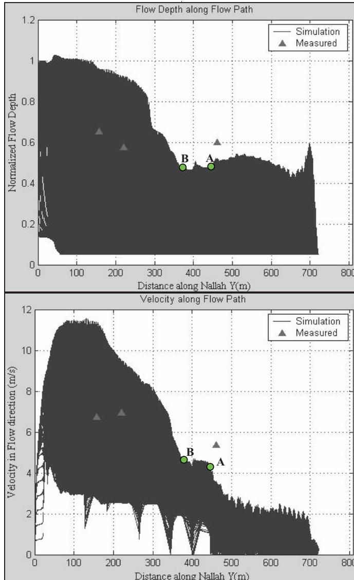
**Fig.15** Flow depth and velocity distribution showing maximum and minimum envelopes along with measured values
