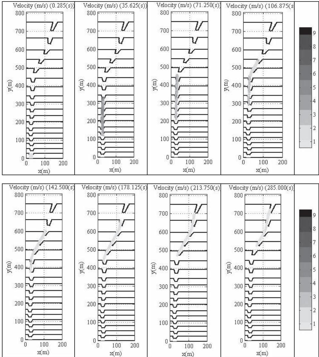
**Fig.14** Velocity (in the direction of flow) distribution along the entire reach of Gulshan Nallah
