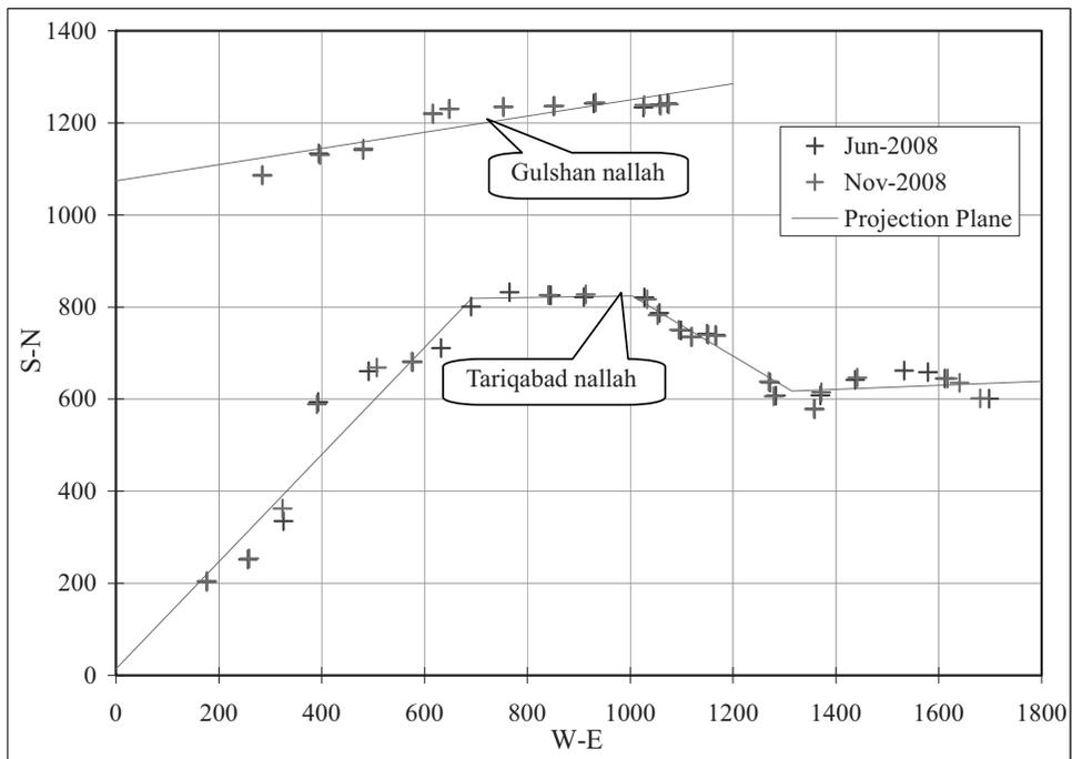
**Fig. 5:** Profiles of Gulshan and Tariqabad Nallahs along with a common projection plane
