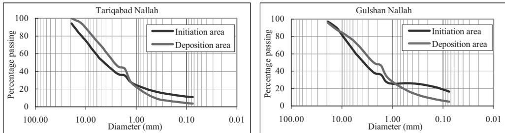
**Fig.12** Grain size distribution of source and deposited material in Gulshan and Tariqabad nallahs
