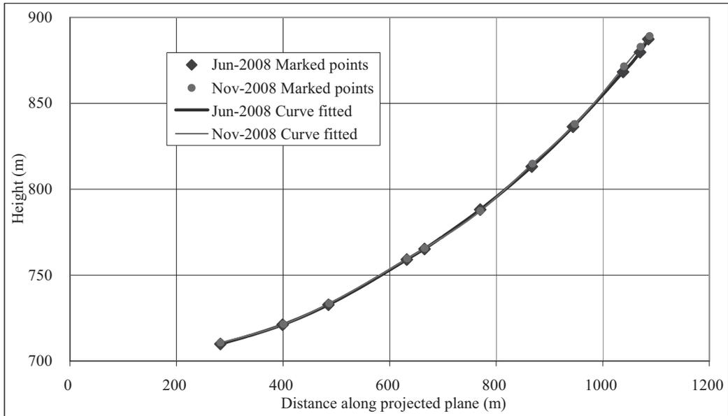
**Fig. 6:** Plot of June 2008 and November 2008 measured data points with curves fitted using cubic *spline* function
