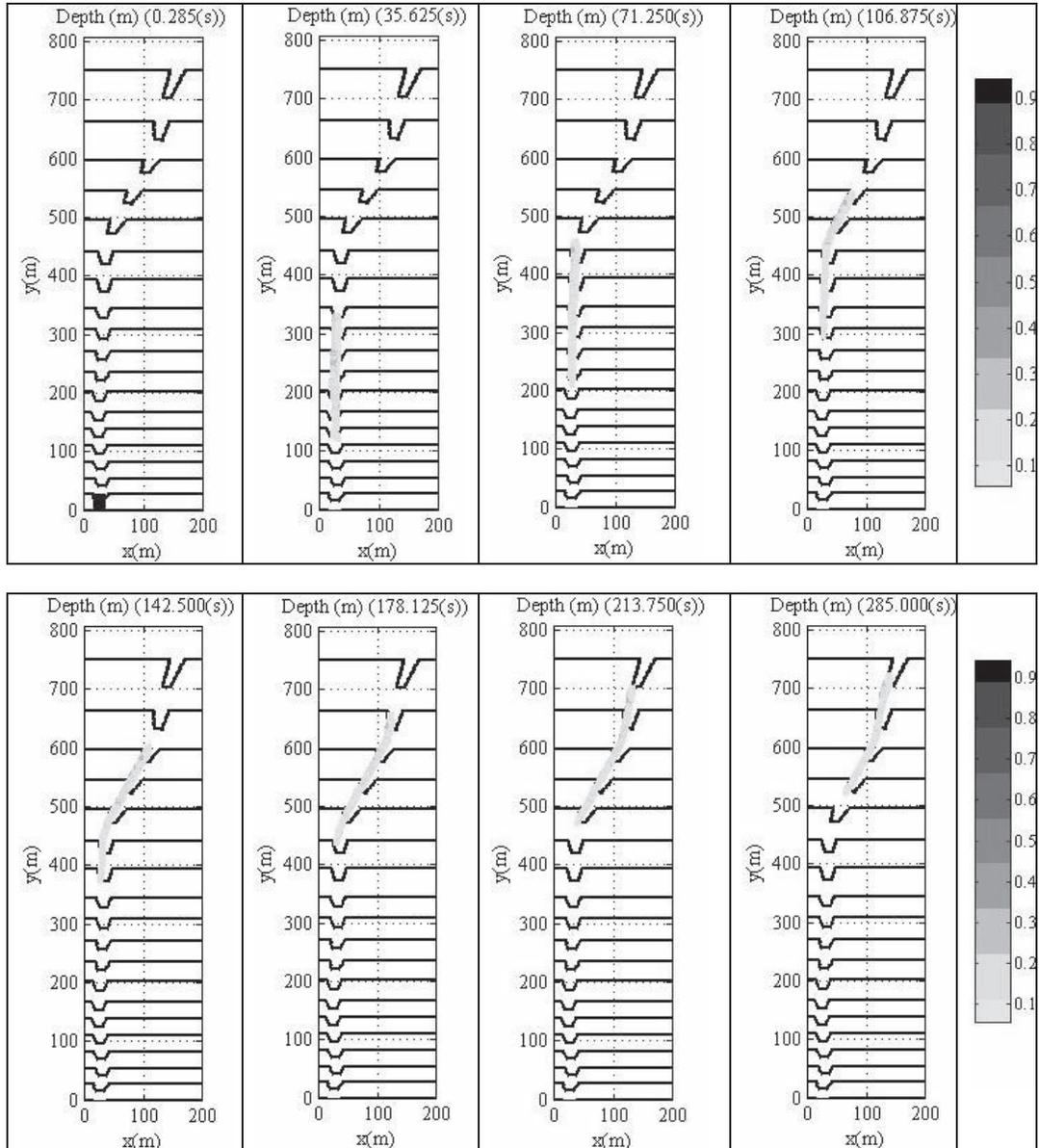
**Fig.13** Flow depth distribution and flow behavior along the entire reach of Gulshan Nallah
