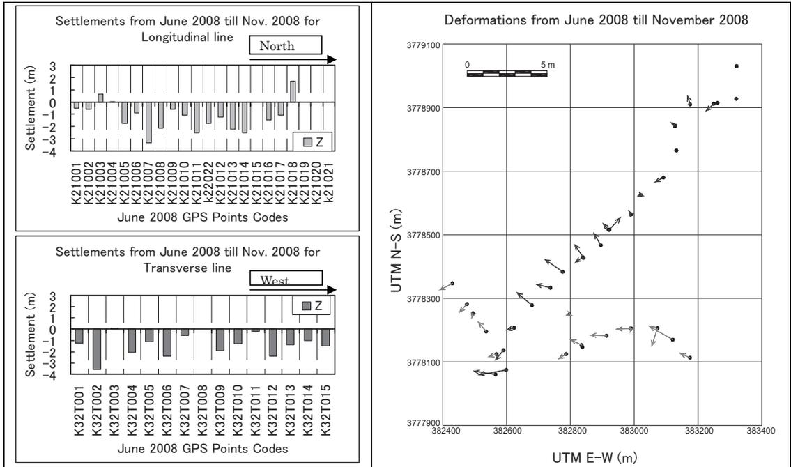
Fig. 11 Results of GPS Data comparison of June 2008 and November 2008. Settlements for Longitudinal and Transverse lines shown on left. Deformation vectors in N-S and E-W UTM coordinate plan shown for each GPS point shown on right.
