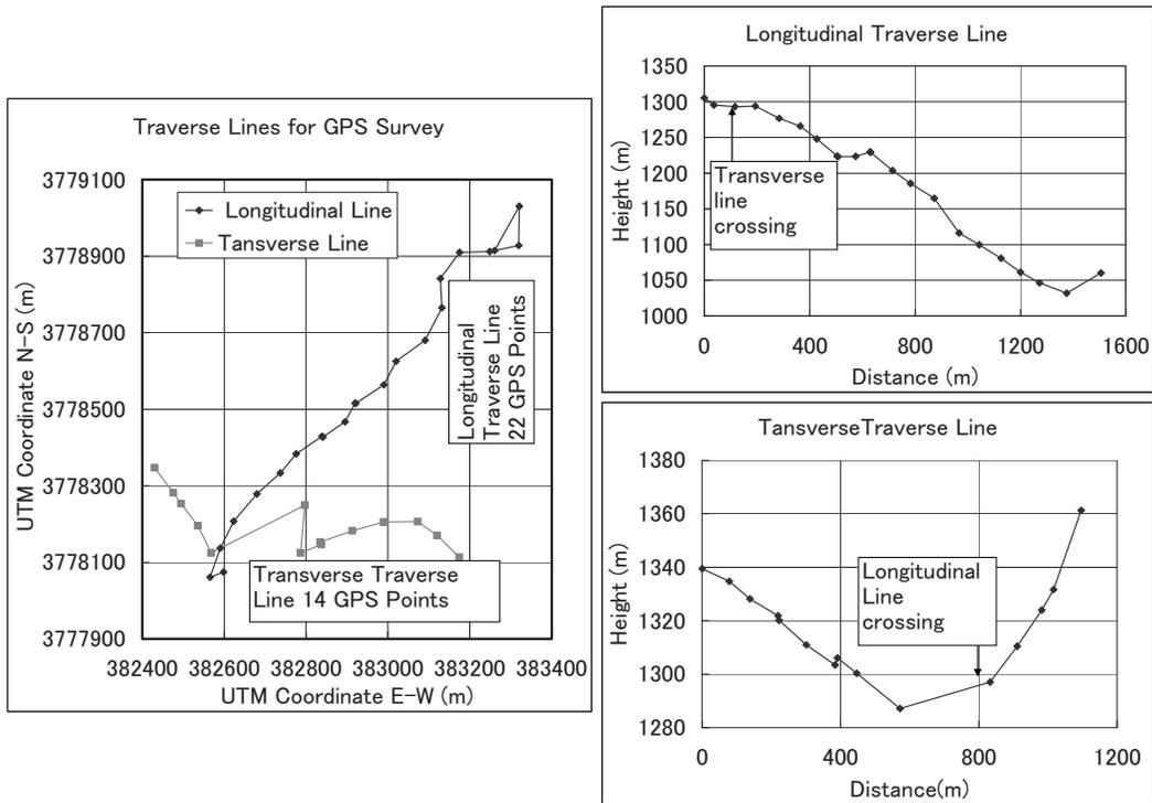
Fig. 9 UTM Coordinates of GPS points. Elevations for Longitudinal and Transverse Traverse lines. (June 2008 Survey Data)
