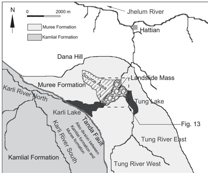
Fig. 2. Schematic map of Hattian Ballah landslide area showing the Tanda fault at south and landslide source scar parallel to the fault. Tanda fault lays the boundary between Kamliyal formation and Muree formation. (Compiled from different sources).
