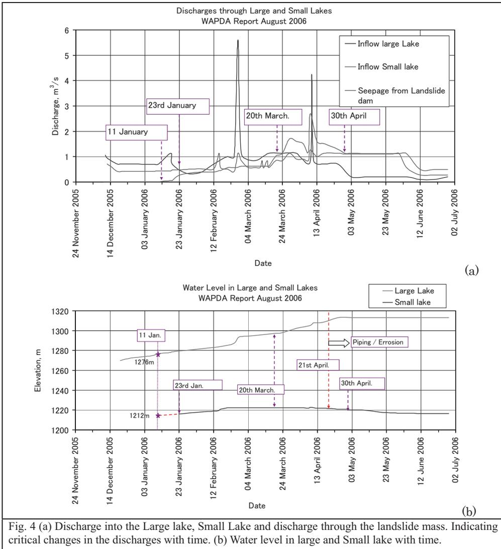
Fig. 4 (a) Discharge into the Large lake, Small Lake and discharge through the landslide mass. Indicating critical changes in the discharges with time. (b) Water level in large and Small lake with time.
