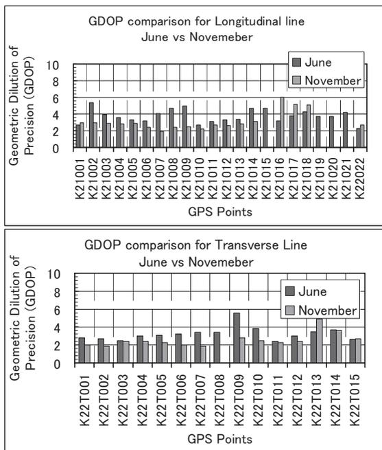
Fig. 10 Geometric dilution of precision for June 2008 and November 2008 surveys. Average of 3.7 and 3.1 for June and November survey respectively for longitudinal lines. Average of 3.0 and 2.5 for June and November survey respectively for transverse traverse line.
