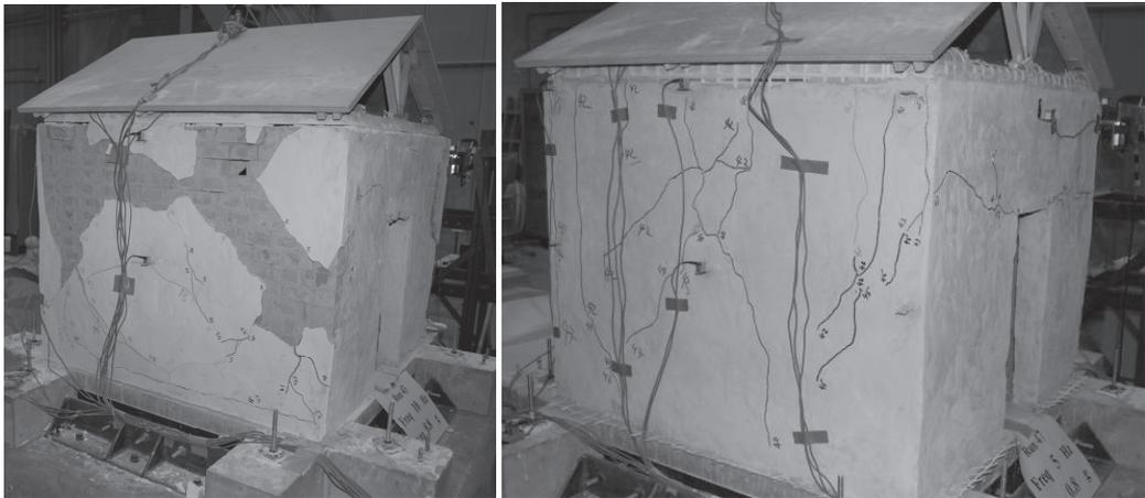
**Figure 7.** Specimen A-4-NR-P after run 43 (left) & Specimen A-4-RE-P after run 48 (right)
