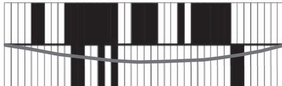
(b) Situation of failed ceiling panels and curving deformation of wooden center frame in gathering room
