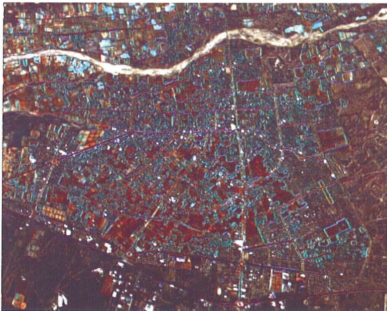
Figure 9. Standard deviation of the twelve pre-event images of Bam City (pseudo color).
