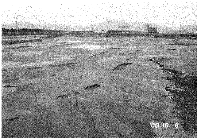
Fig. 9 Sand boils at Sakai Minato dream port park
