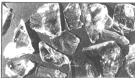
Figure 1 Micrographs of the glass grains at a magnification of 10 times. After close examination of a single grain, hackle and rib marks can be observed.
