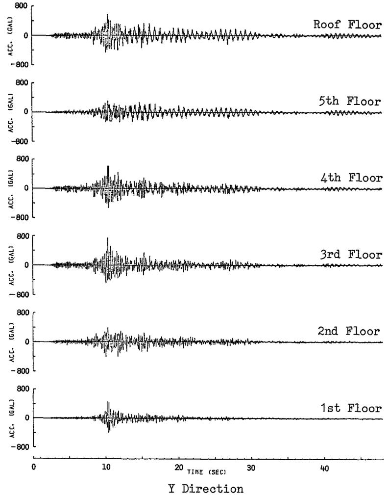
Fig. 8 Time histories of Acceleration of Weak Column Structure
