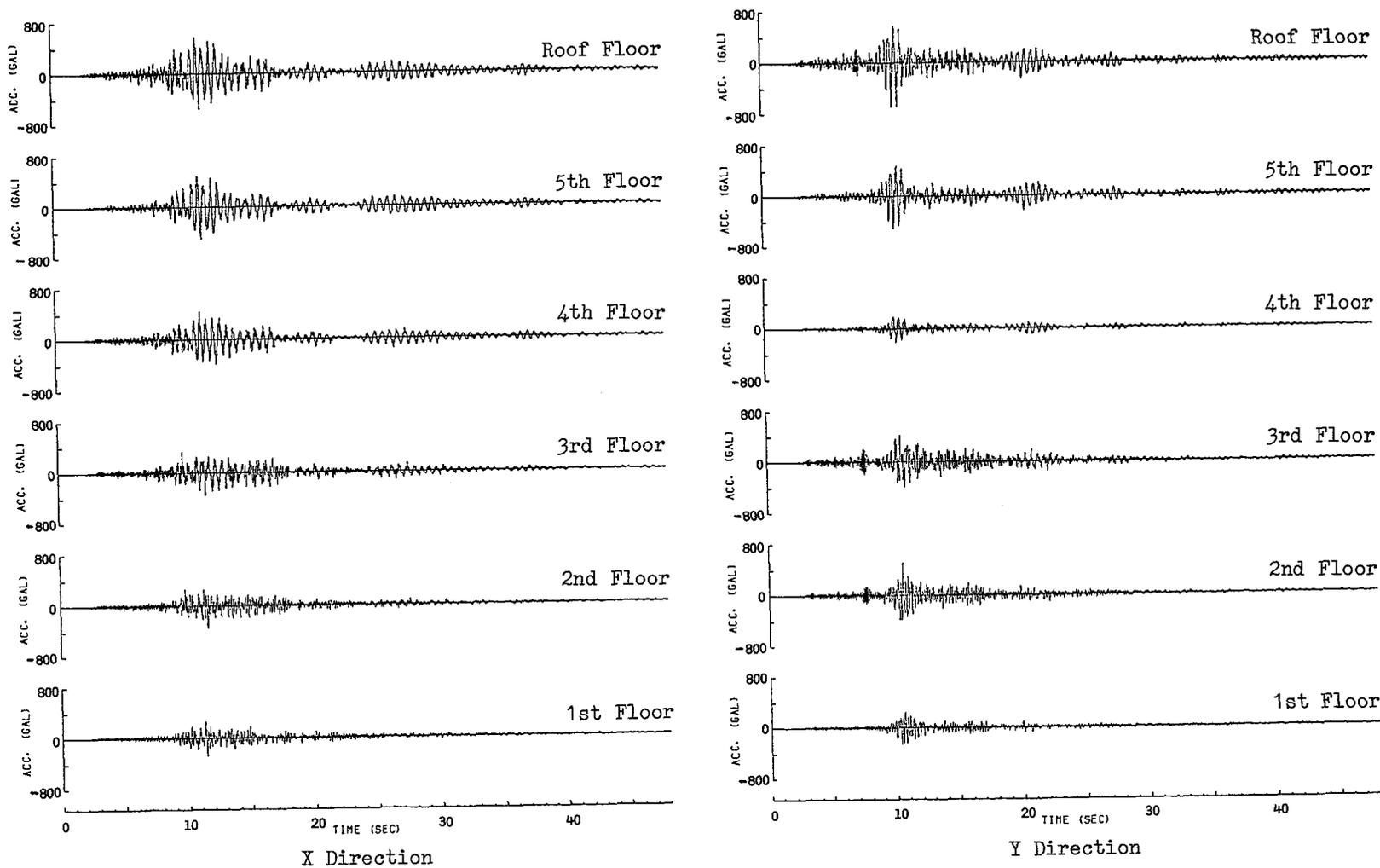
Fig. 12 Time Histories of Acceleration of Weak Beam Structure
