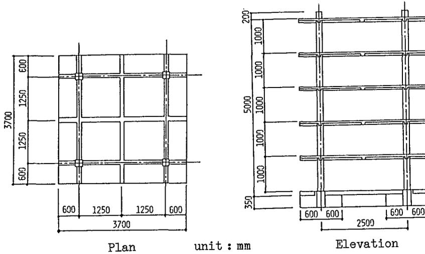
Fig. 1 Plan and Elevation of Weak Model Structure
