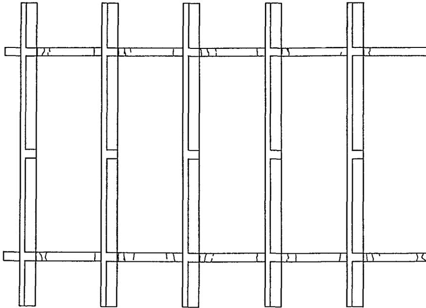
Fig. 7 Crack Patterns of Weak Column Structure
