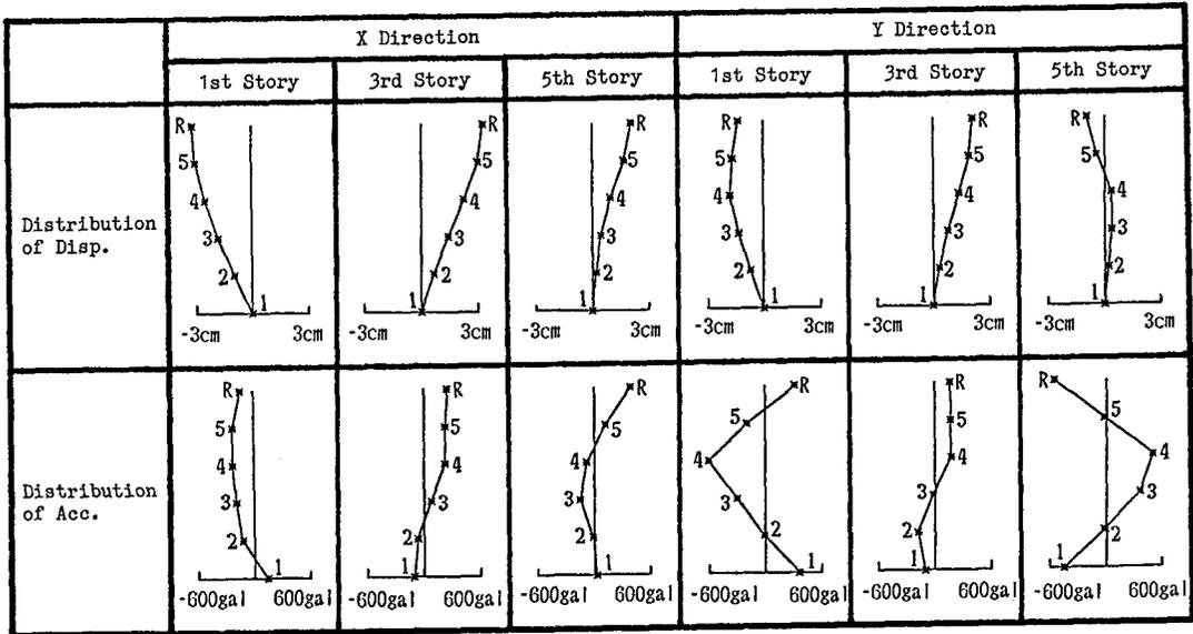
Fig. 9 Distribution of Displacement and Acceleration of Weak Column Structure
