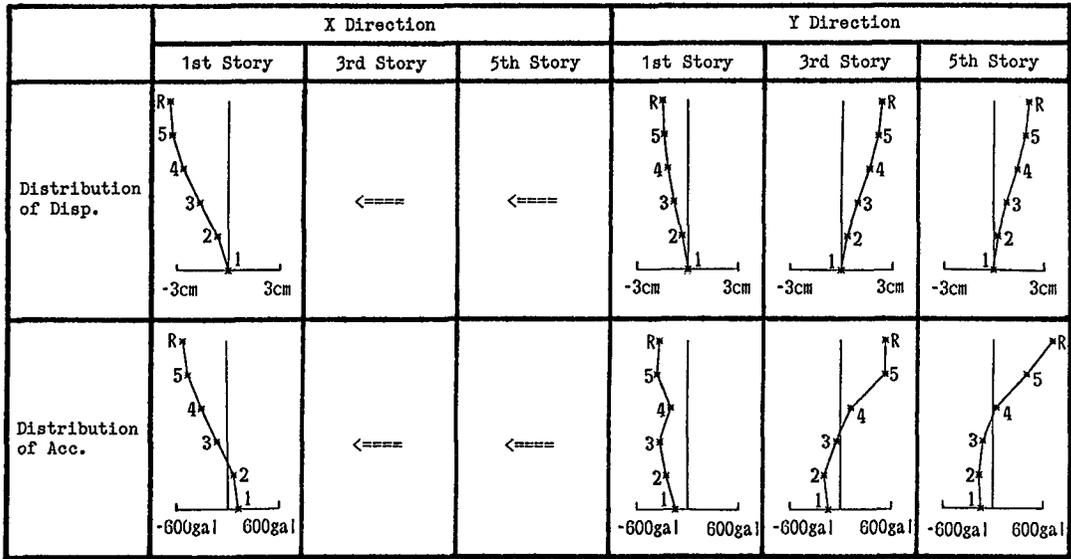
Fig. 13 Distribution of Displacement and Acceleration of Weak Beam Structure
