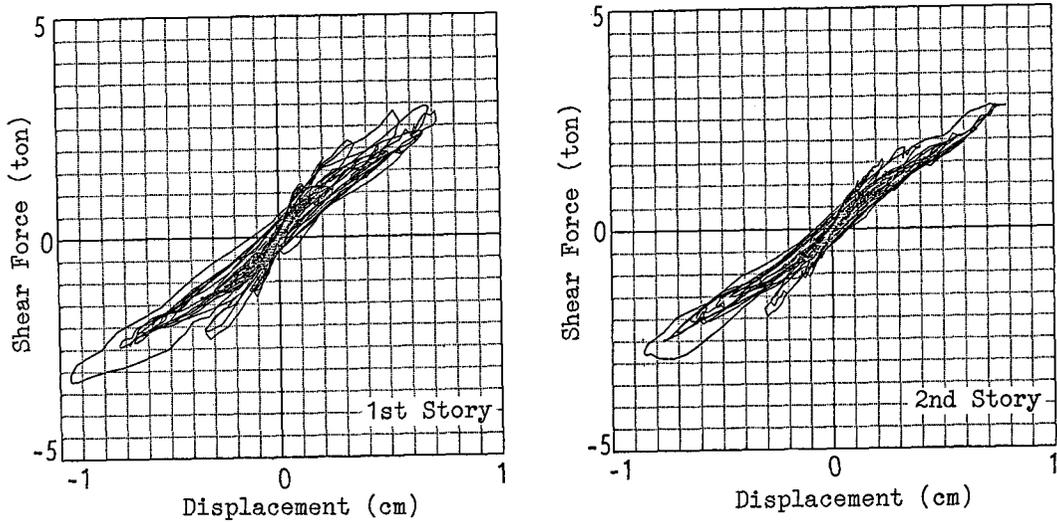
Fig. 10 Hysteresis Loops of Weak Column Structure at 1st and 2nd Story in X Direction
