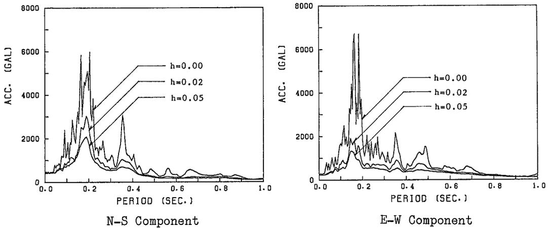
Fig. 6 Response Acceleration Spectra of Ground Motion
