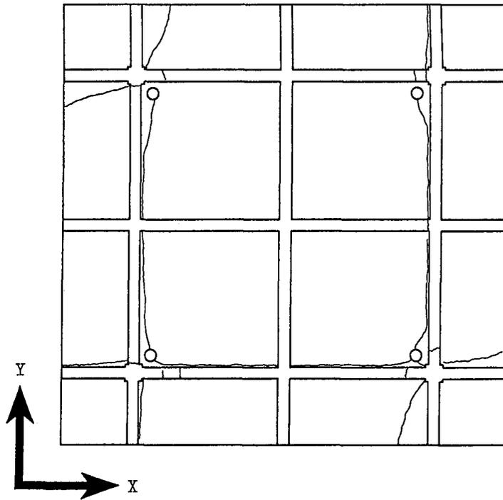
Fig. 11 Crack Patterns of Weak Beam Structure at 3rd Floor System
