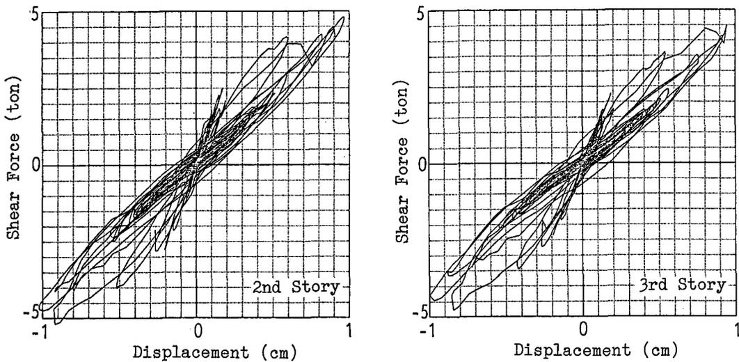
Fig. 14 Hysteresis Loops of Weak Beam Structure at 2nd and 3rd Story in X Direction
