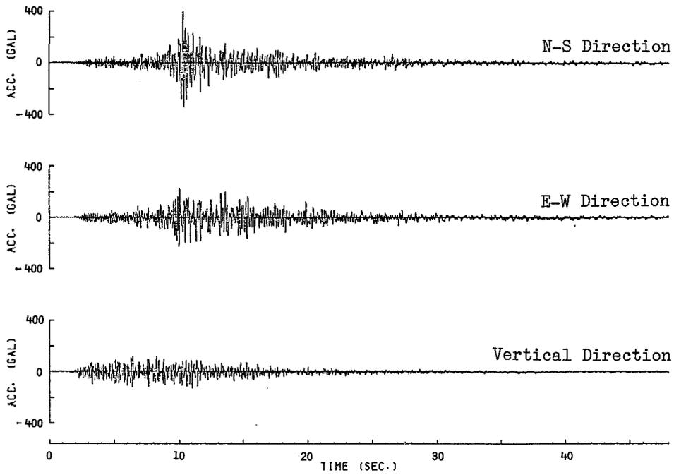
Fig. 5 Time Histories of Acceleration of Ground Motion
