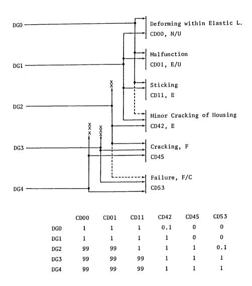
Fig. 12A) State Trasition Chart and Conversion Matrix.
