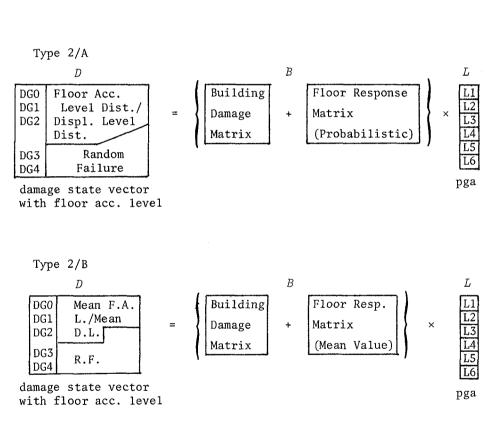
Fig. 1 Schematic Relations Input Peak Ground Acceleration Vector to Damage State Vector
